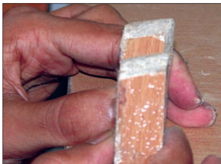
File the wood leg to give the required tilt
