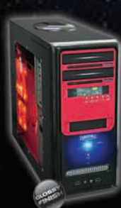
Antibiotic Front LCD display Transparent side panel Side 80mm & 120mm LED fans, Toolfree
