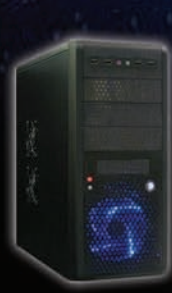
Bijli Perforated front panel 120mm front fan Two 80mm fans on side
